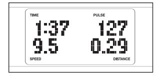
The lower left corner of the display will show your pedaling speed, in miles or kilometers per hour.
